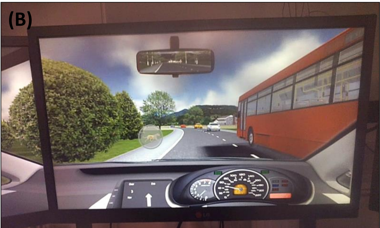
Figure 2: Panel A shows the three-screen Carnetsoft simulator. The participant is wearing the SMI eye tracking glasses. Panel B shows a screen shot of the central screen as hazard 1 triggers (see Table 3 for a list of hazards). This image is taken from the camera of the eye tracking glasses, and the grey circle represents the participant's fixation on the dog entering the road.
