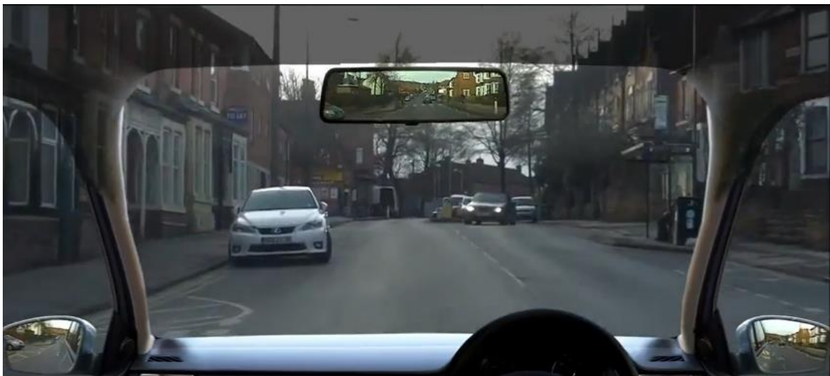
Figure 3. A hazard prediction clip typically occludes just as the hazard begins to develop. This screen shot is taken just before occlusion and shows an oncoming vehicle that is about to turn across your path.
