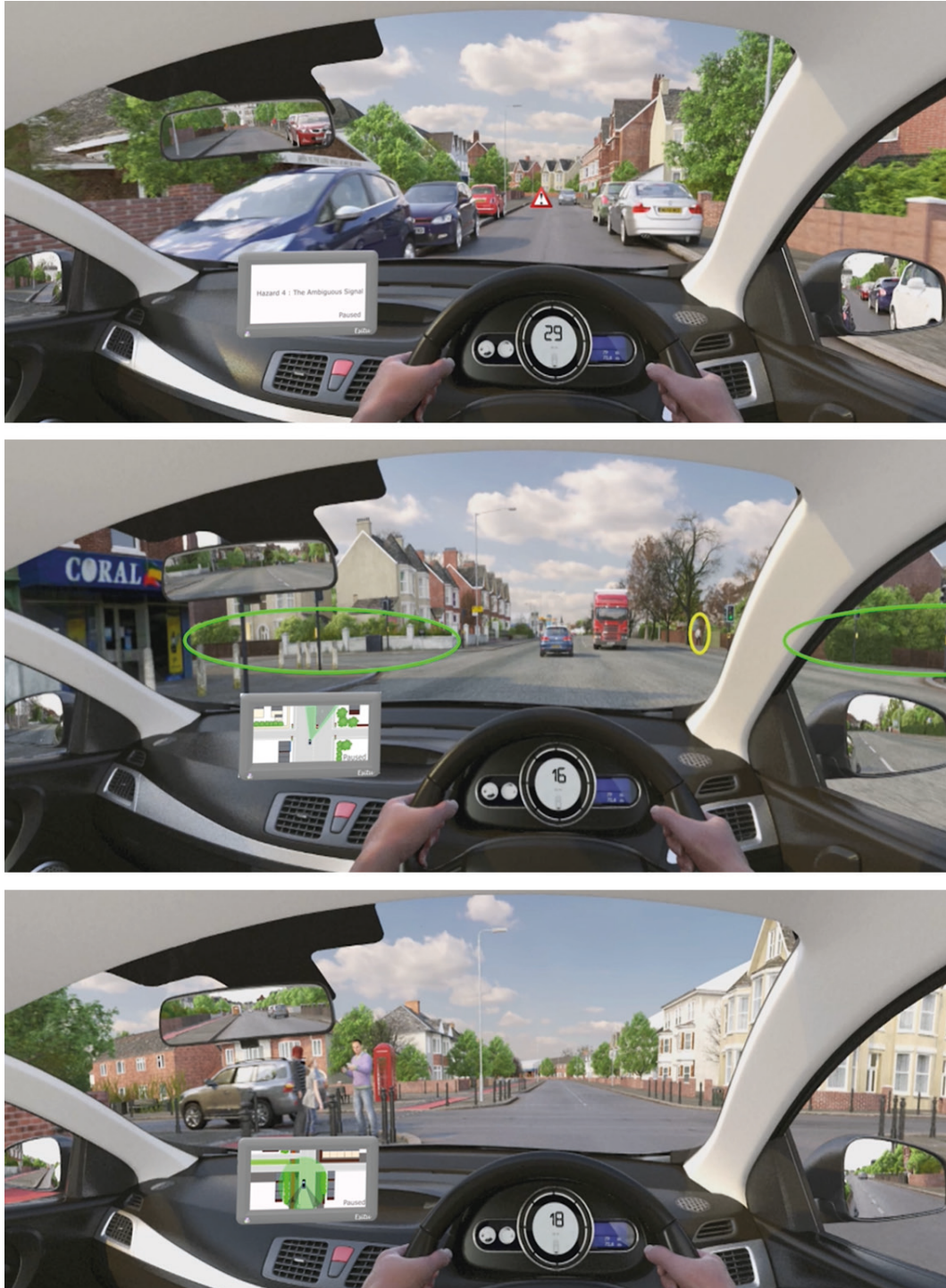
Figure 5.1: Three screenshots showing different forms of visual feedback in Study 4: a warning symbol (top panel), the use of ellipses to indicate where drivers should look (middle panel), and the use of a virtual satnav to provide alternative perspectives on hazards (middle panel and bottom panel)
