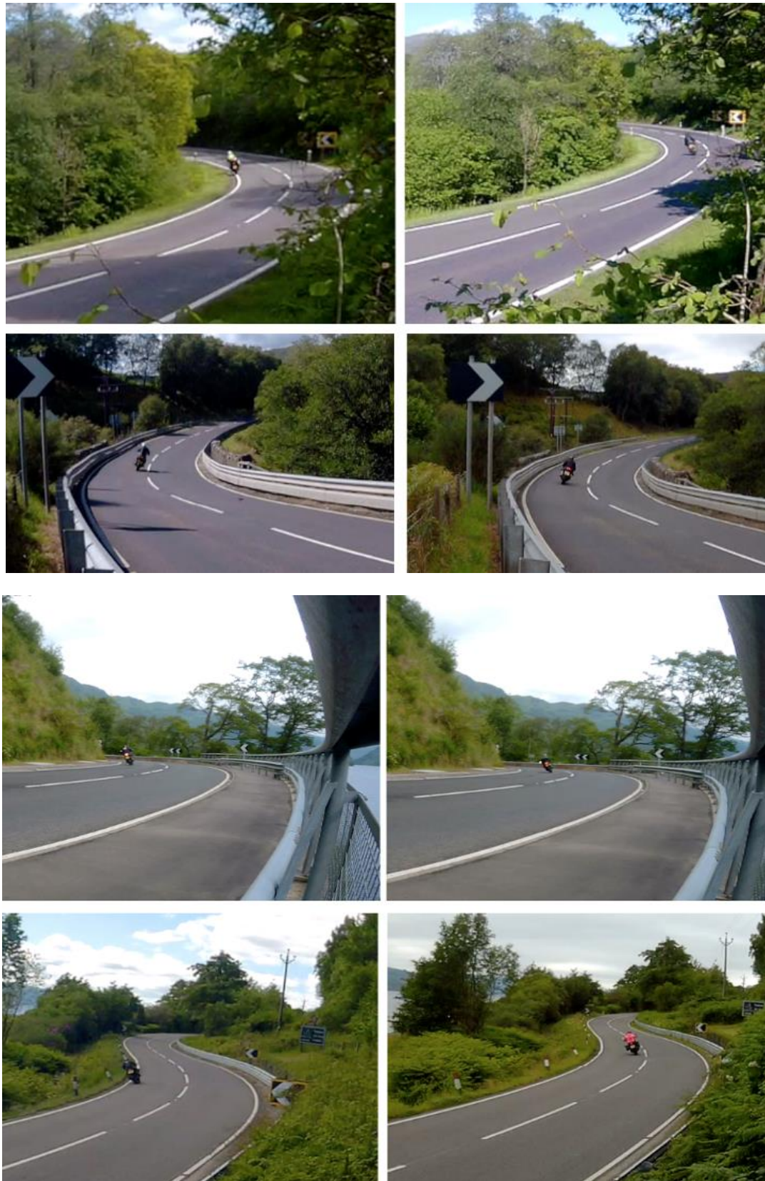
Figure 4: Changes in road position (left-hand images = without PRIMEs installed, right-hand images = with PRIMEs installed)
